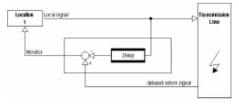
After being removed from the returning broadcast signal, the local source can be directly added again. The volume of this direct signal is adjustable, and it is added automatically when a return signal is present.
