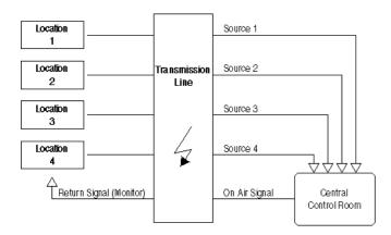
The Echo Canceller has been designed to overcome problems in live broadcasting, when transmission delays due to digital transmission and data compression processes do not allow using the broadcast signal as monitoring source.
